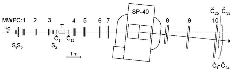
**Fig. 1.** Layout of the spectrometer.
