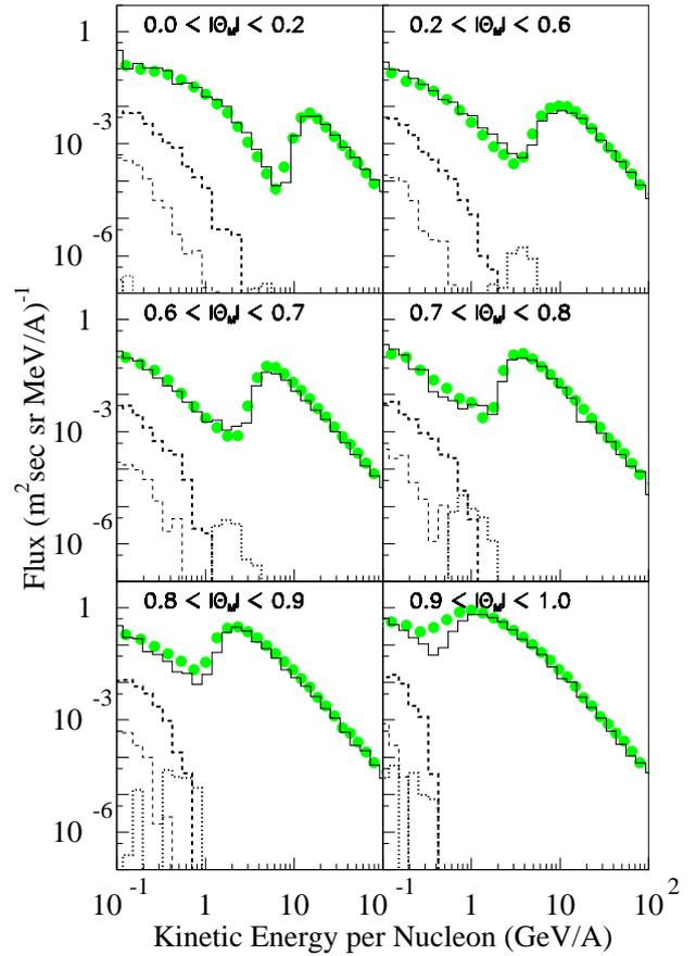
**Fig. 1.** Simulated spectra for downward  $p$ (primary+secondary) (solid lines),  $D$  from fragmentation (dotted lines), coalescence  $D$  (dashed thick lines),  ${}^3\text{H}$  from coalescence (dashed thin lines) separate according to the CGM latitudes ( $\theta_M$ ). Full circles correspond to the experimental  $p$  spectra measured by AMS (J. Alcaraz et al., 2000a).
