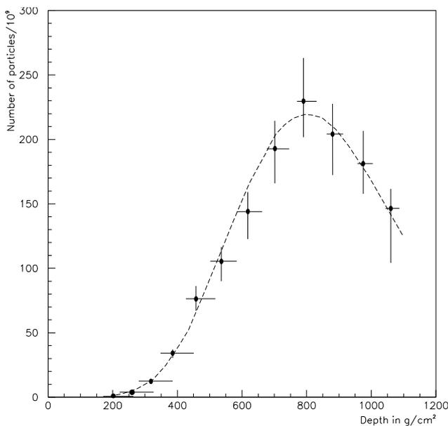
**Fig. 3.** Reconstructed shower longitudinal profile for the highest energy Fly's Eye event (Bird et al., 1995)
