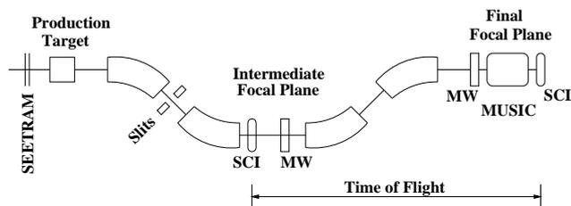
**Fig. 1.** Schematic layout of the FRS fragment spectrometer. Fragments are separated by the four large dipole magnets. Scintillators (SCI) measure the time of flight over the second half of the spectrometer as well as the horizontal beam position. Multi-wire chambers (MW) are used for beam tuning and removed for production measurements.
