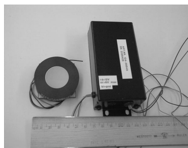
Fig. 6. A 73-pixel HPD (left) with 12 kV power supply (right).
