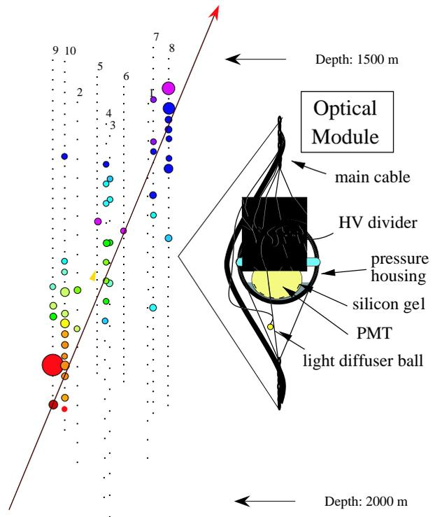
**Fig. 1.** The AMANDA-B10 detector as of 1997. Each dot represents an optical module. The modules are separated by 20m on the inner strings (1-4), and by 10m on the outer strings (5-10). Shown is an experimental neutrino event. The size of the circles indicates the amplitude of each detected signal the color indicates the time of the photon's arrival. Earlier times are in red, later in blue. The arrow indicates the reconstructed track of the up-going muon.
