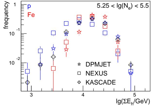
**Fig. 4.** Frequency distribution of the hadronic energy sum  $\Sigma E_h$ . The electron number bin corresponds to a primary energy of about 1.5 PeV for proton and 5 PeV for iron induced showers. The QGSJET distributions, not plotted here, are similar to DPMJET.
