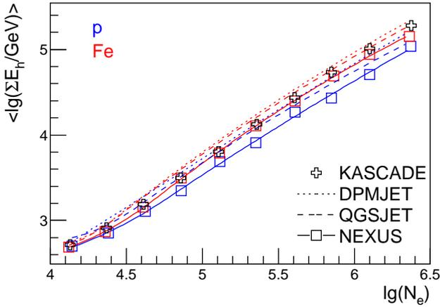
**Fig. 2.** Hadronic energy sum  $\Sigma E_h$  versus electron number  $N_e$ . For QGSJET and DPMJET only the parameterizations are plotted. The electron number range  $4.0 < \lg N_e < 6.5$  corresponds to a primary energy range 0.3–20 PeV for proton and 0.5–40 PeV for iron induced showers. NEXUS predicts too few hadrons at constant electron numbers.
