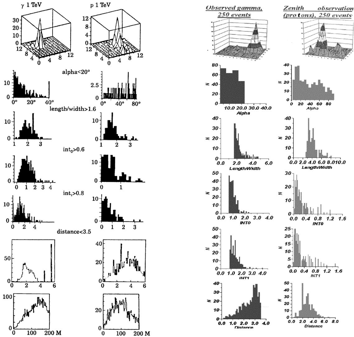
**Fig. 1.** Monte Carlo distribution of image parameters for gamma-quanta and protons showers of 1 TeV and experimental SHALON distribution of image parameters for gamma-quanta and proton showers with energy more than 0.8 TeV
