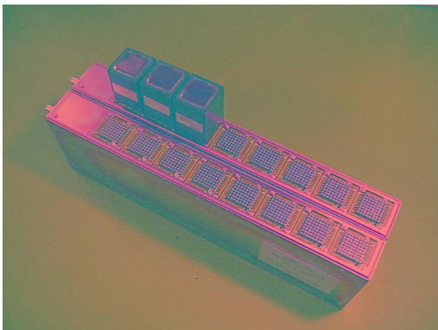
**Fig. 6.** Two units of MA-PMT readout system. The unit contains 16 pairs of VA32\_hdr2 and TA32cg, and 512 SCIFIs can be read with one unit.
