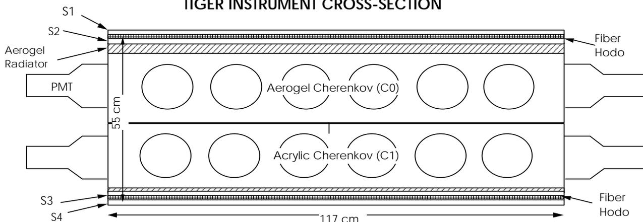
**Figure 2.** A cross-section of the TIGER Detector. S1 and S2 are the top scintillator detectors, S3 and S4 are the bottom scintillation detectors. The TIGER instrument is about 117 by 117 cm square and 55 cm high.
