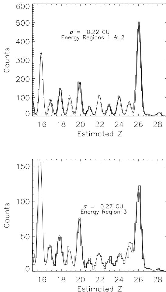
**Figure 1.** Charge Resolution for the 1997 TIGER instrument, which flew for one day out of Ft. Sumner New Mexico. The top plot shows the charge resolution for particles with energy less than 4.3 GeV/nucleon. The bottom plot shows the resolution for particles with energy greater than 4.3 GeV/nucleon. We expect to obtain better charge resolutions for the TIGER 2001 instrument.
