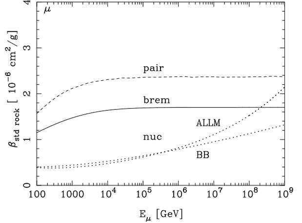
Fig. 1. Contributions to Muon energy loss.
