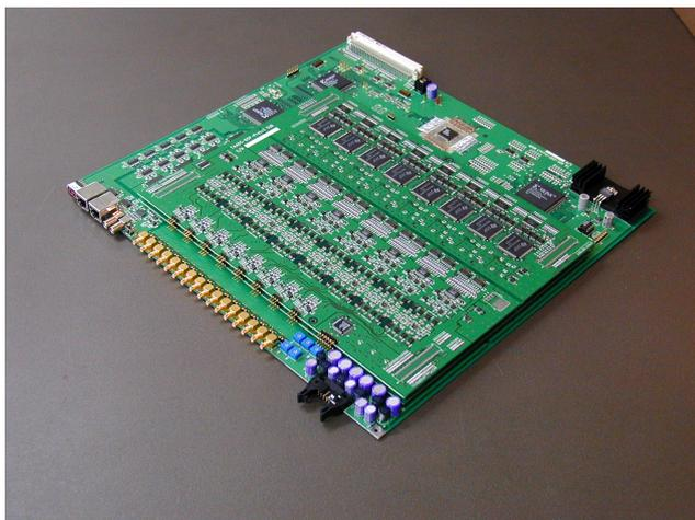
**Fig. 6.** Proto-3 module of signal finder. The height of the module is 9U but the depth of the module is extended to 50 cm.
