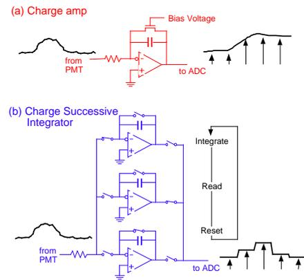
**Fig. 3.** Schematics of Charge Successive Integrator.
