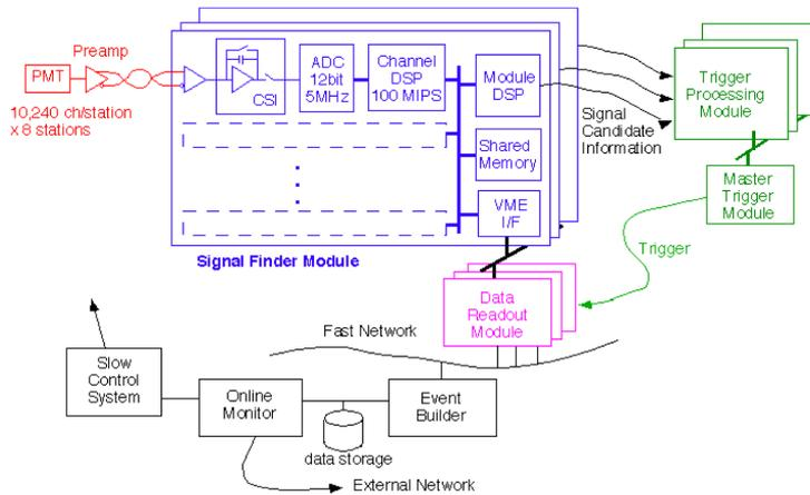
**Fig. 2.** Block diagram of the TA online system.
