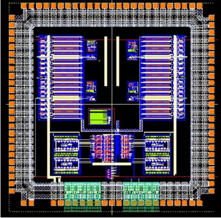
**Fig. 4.** Layout of the test CSI cell designed in  $0.6 \mu\text{m}$  CMOS technology.
