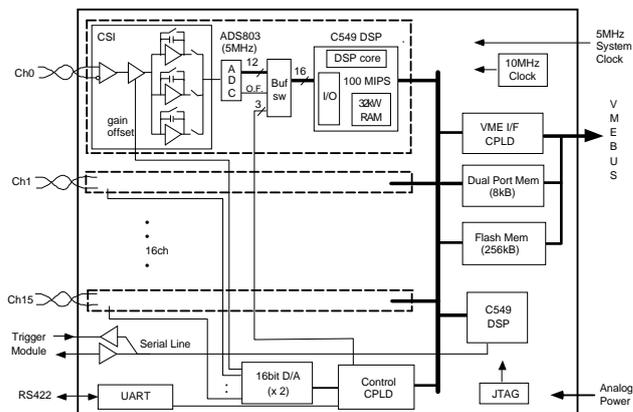
**Fig. 7.** Block diagram of the 16-ch prototype Signal Finder module. The module is implemented in a 9U VME board.
