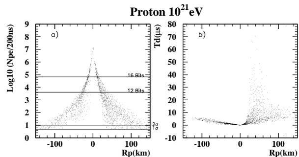
**Fig. 1.** Maximum number of photoelectrons per 200 ns time bin for one PMT versus impact parameter  $R_P$  of the event (left). Signal duration versus  $R_P$  for the same PMT (right). The sign of  $R_P$  distinguishes between going (plus) and coming (minus) tracks of observed air-shower events with respect to a detector station.
