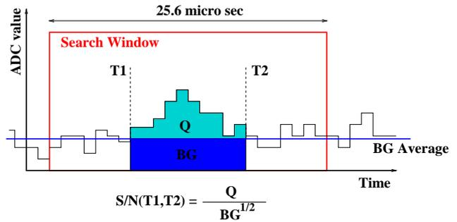
**Fig. 5.** Signal finding algorithm.
