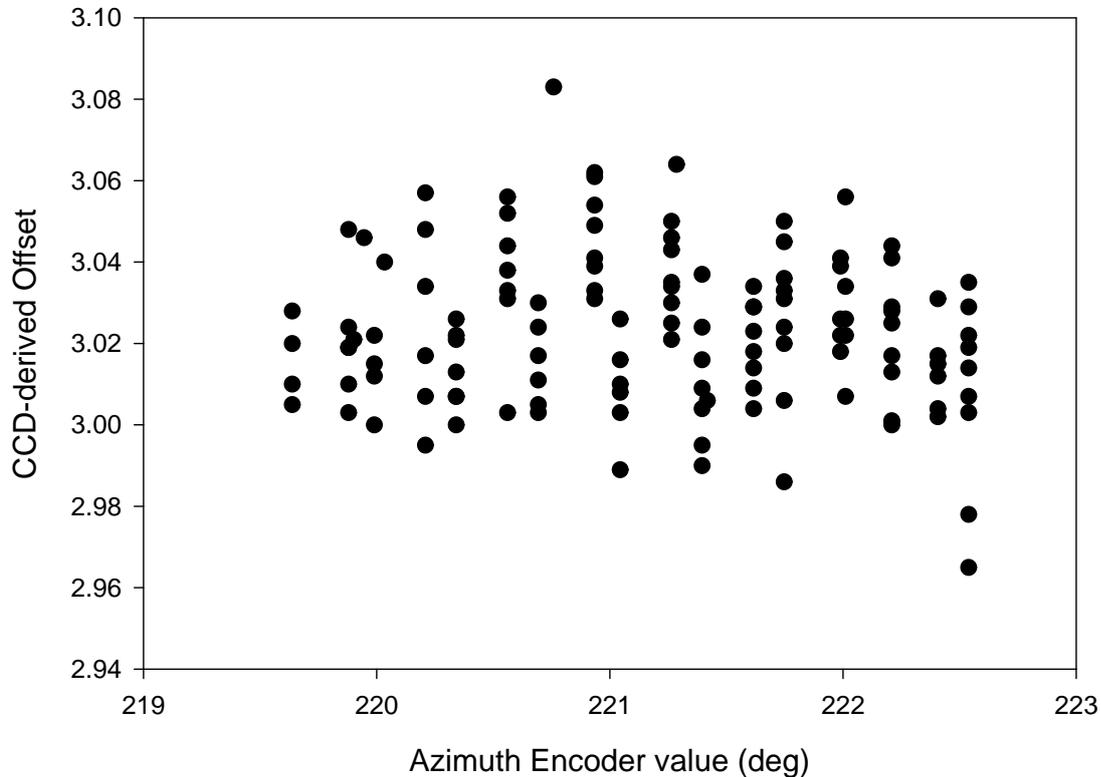
**Fig. 1.** The difference between the azimuth encoder values and the predicted position of the source being tracked, in degrees, as a function of time during a sample 15-minute run. The offset of  $\sim 3$  degrees was intentional.
