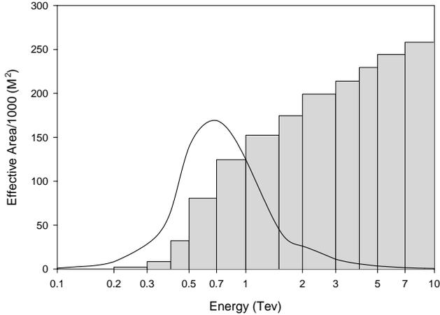
**Fig. 5.** The histogram gives the variation of the effective area of the telescope with energy for gamma ray showers. The curve, having a vertical scale in arbitrary units, shows the form of the triggering spectrum for a power law differential source energy spectrum of index -2.6.
