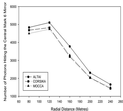
**Fig. 1.** Plot of Mean Number of Photons Hitting a Central Mark 6 Mirror, with atmospheric absorption, for a US Std Atmospheric Profile at an altitude of 1800 metres for a 1TeV Photon Primary for ALTAI, CORSIKA and MOCCA at fixed radial distances.
