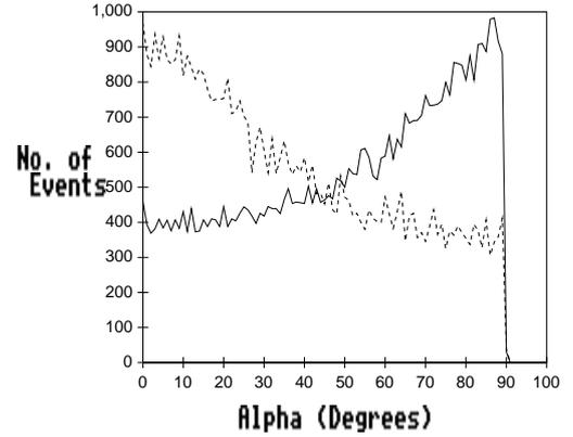
**Fig. 4.** Plot of ALPHA for real off source (cosmic ray) data (solid) versus simulated gamma data (dotted)
