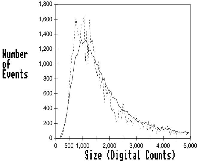
**Fig. 3.** Plot SIZE (in digital counts) versus number for real cosmic ray events (solid) and simulated cosmic ray events (dotted).
