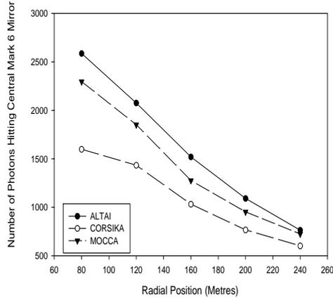
**Fig. 2.** Plot of Mean Number of Photons Hitting a Central Mark 6 Mirror, with atmospheric absorption, for a US Std Atmospheric Profile at an altitude of 1800 metres for a 1TeV Proton Primary for ALTAI, CORSIKA and MOCCA at fixed radial distances.
