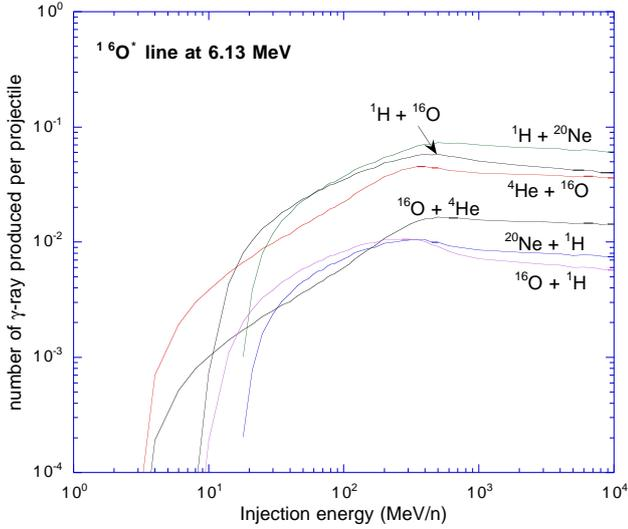
**Fig. 2.** Absolute photon yields,  $\mathcal{N}_{i,j;\gamma}$ , in the 6.13 MeV line of  $^{16}\text{O}$  through various channels, as a function of the injection energy of the projectile. The latter is the first nucleus appearing in the label, and the target is the second.
