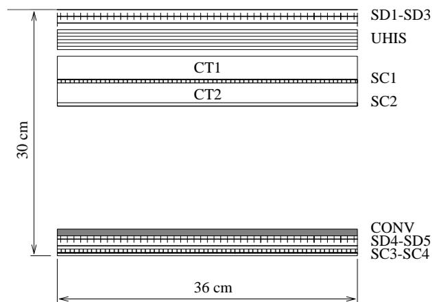
**Fig. 2.** The schematic layout of the KLEM device for the NUCLEON mission.
