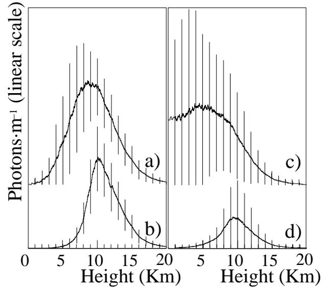
**Fig. 2.** Average number of Cherenkov photons generated per unit length of atmosphere depth for  $\gamma$ -showers (a) and protons (c). For curves b) and d) only those photons within the restricted field of the heliostats in convergent view (core position at the center of the array) have been counted. The error bars are the  $1 \sigma$  deviations of the photon yield distribution at the corresponding height.
