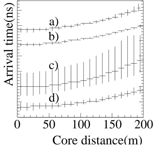
**Fig. 4.** Cherenkov front shape for 200 GeV  $\gamma$ -rays (a, b) and 500 GeV protons (c, d) as seen with a unrestricted field of view (a, c) and with a restricted field and convergent view (b, d).
