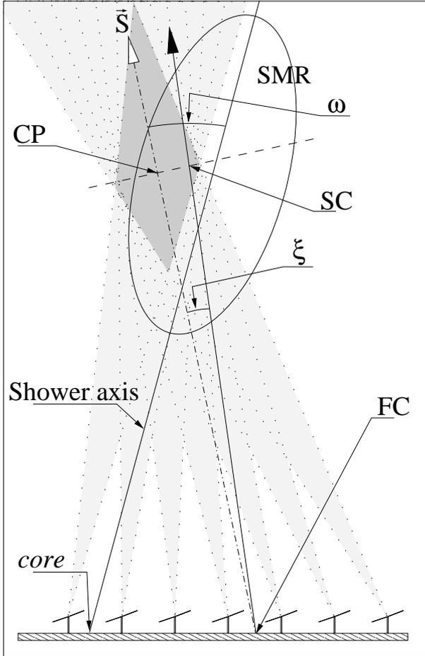
**Fig. 1.** Schematic view of a shower detected with a heliostat field pointing to  $S$  in convergent view. The heliostats aim at the convergent point CP. Only a fraction of the SMR is observed. The reconstructed direction is determined by the sphere center SC and the field center FC.
