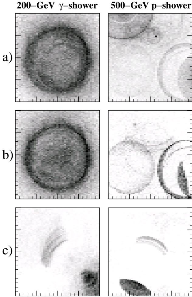
**Fig. 3.** Spatial distribution of Cherenkov photons in a square of  $300 \times 300 \text{ m}^2$  at ground (500 m a.s.l.) for both a 200 GeV  $\gamma$ -ray shower and a 500 GeV proton shower. a) All photons are plotted (NRFV); b) Only those photons detected by a restricted field/convergent view array (RFCV with  $r = 0$ ); c) the same as b) but with the shower axis shifted by about 60 m.
