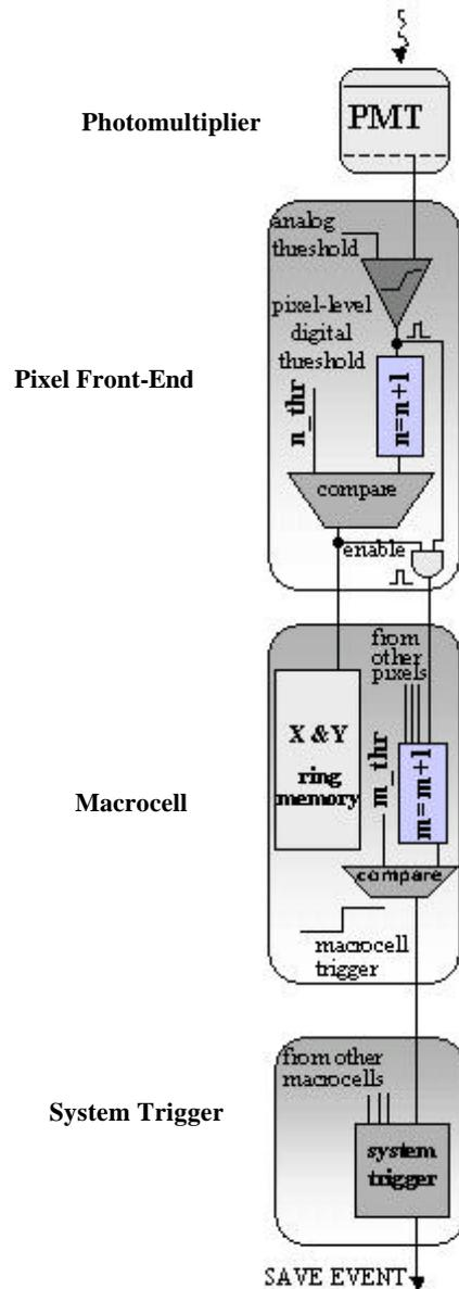
**Fig.4.** Functional block diagram of the EUSO system electronics.
