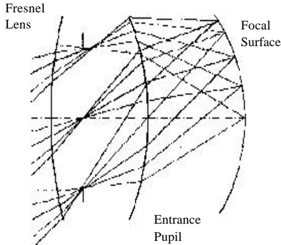
Fig. 2. Ray tracing of doubled curved Fresnel lens focusing the light on the curved focal surface.
