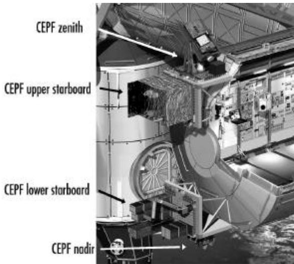
**Fig. 5.** An artist's impression of the CEPF on a cutaway view of the Columbus module. The four positions are indicated, and typical payloads are shown.
