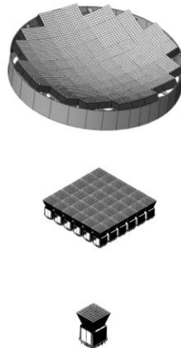
Fig. 3. Schematic representation of photomultiplier + light collector (bottom), macrocell (middle), focal surface photo-detector (top).
