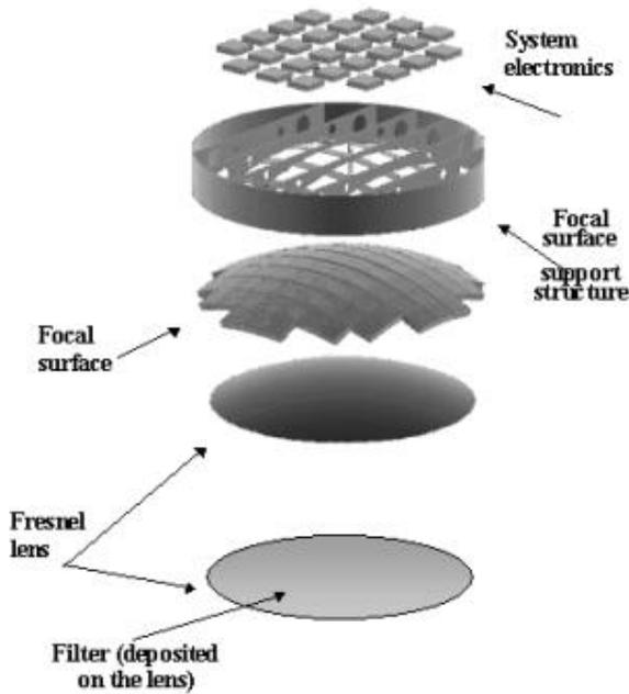
Fig. 1. Exploded artistic view of the EUSO telescope.
