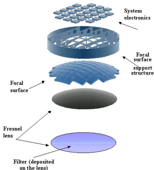
Fig.2. Exploded artistic view of the *EUSO* telescope.
