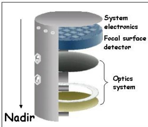
**Fig.4.** Scheme of the *EUSO* main telescope.
