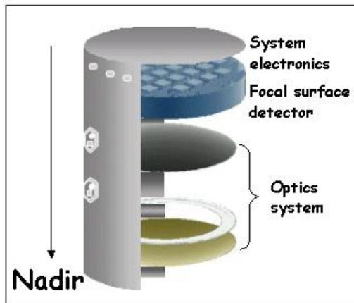
**Fig.4.** Scheme of the *EUSO* main telescope.
