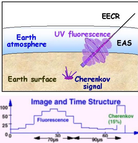
Fig.1. Time profile of the emitted UV light from an EAS.
