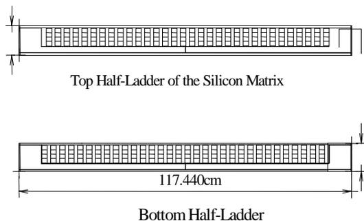
**Fig. 2.** This figure shows two motherboards that make up a ladder of the silicon matrix. The top half-ladder is inverted and placed over the bottom half-ladder so that the detectors are offset by half a pitch. The detectors are spaced so that they slightly overlap within the ladder. This makes the ladder continuously sensitive over its length.
