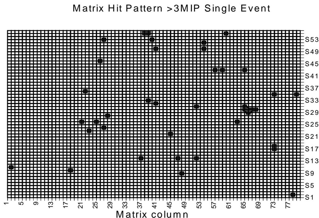
**Fig. 3** This figure shows the pattern of hits in the silicon matrix from a single event. Each grid intersection corresponds to a single pixel in the matrix. This event has a deposited energy in the calorimeter of 87 TeV. The hit threshold is 3 MIPs, the typical dividing line between protons and helium.
