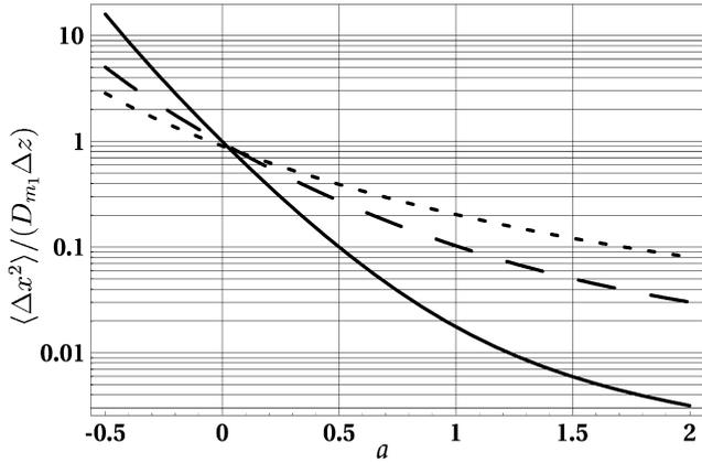
**Fig. 2.** Ratio of the quasilinear field line spreading over the original, diffusive quasilinear prediction for a given value of  $P_{x_{\parallel}}(k_1)$ . Continuous line:  $k_1 \Delta z = 0.01$ . Long-dashed line:  $k_1 \Delta z = 0.1$ . Short-dashed line:  $k_1 \Delta z = 0.3$ .
