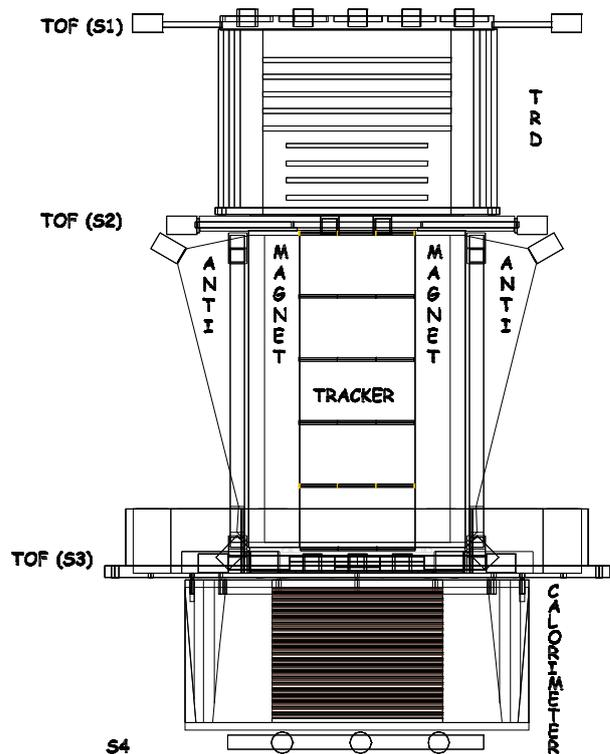
Fig. 1. Schematic view of PAMELA instrument.
