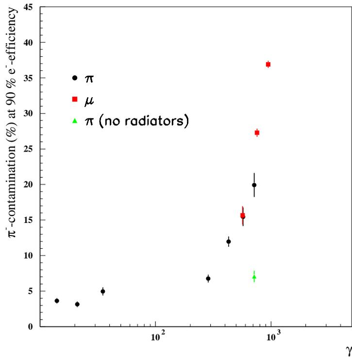
**Fig. 5.** Contamination from pions and muons at 90% electron efficiency versus the Lorentz factor  $\gamma$ .
