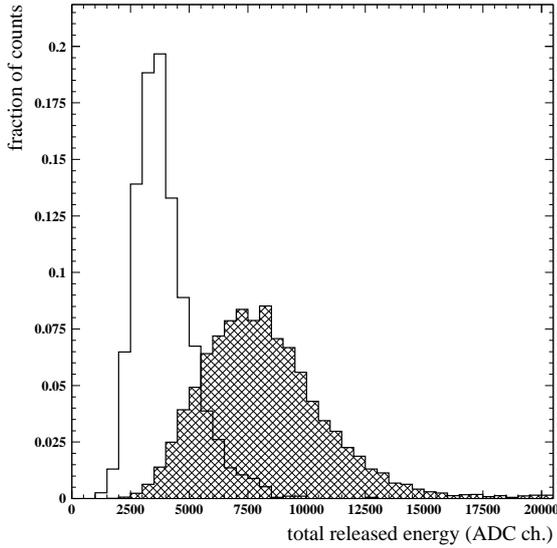
**Fig. 3.** Total energy detected in the TRD for radiating (electrons) and non-radiating (pions) particles of 40 GeV/c momentum.
