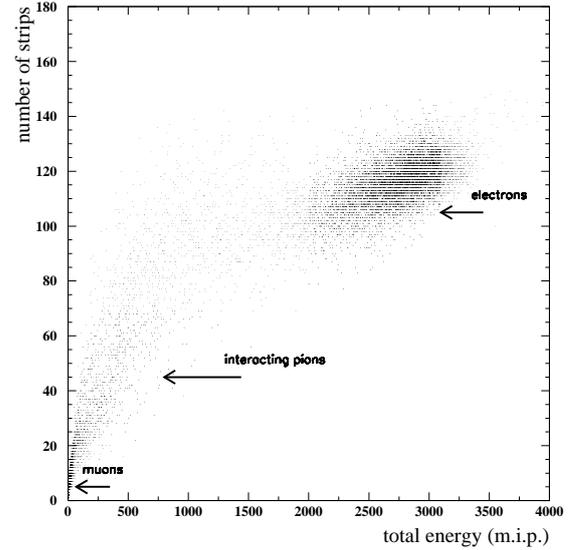
**Fig. 4.** Particle selection with the calorimeter: the discriminating variables are shown for particles at 80 GeV/c. The three event sets used for this data analysis are marked.
