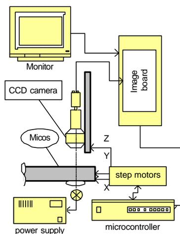
Fig. 1. The setup of CCD based automatic system.
