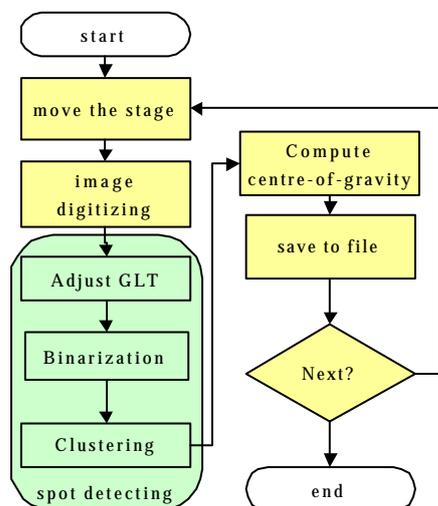
Fig. 2. The flowchart of an automatic scanning system.
