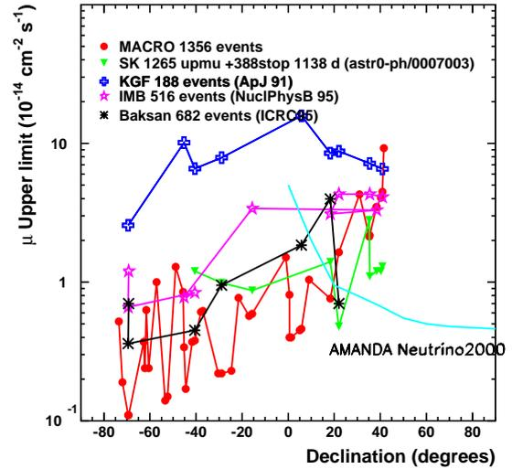
**Fig. 4.** MACRO 90% c.l. upward-going muon flux limits as a function of the declination of 42 selected sources (full dots). Other experiments limit for some sources are shown. All symbols are linked by solid lines to guide the eyes. The limits from AMANDA (Andres, 2000) cannot be directly compared to other experiments in this plot due to the much higher energy threshold.
