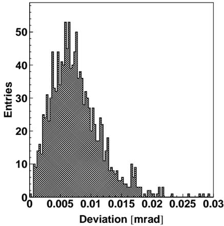
**Fig. 4.** Distances between the nominal position and the one reached after completion of a measurement cycle. The rms deviation is 0.008 mrad. Errors in the mirror alignment are twice the errors of this experiment since the reflection doubles the angle.
