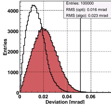
**Fig. 5.** Simulated alignment accuracy for a mirror with a distance of 6 m to the center of the dish. Open histogram and solid vertical line: distribution and worst case for the theoretical optimum. Filled histogram: distribution of the best algorithm found.
