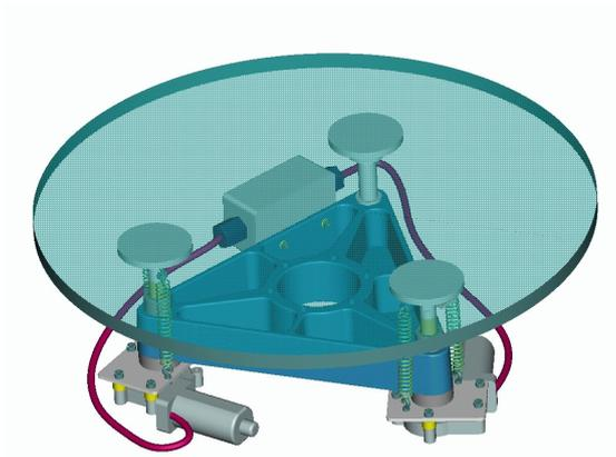
**Fig. 2.** Mounting system with actuators for the mirror adjustment.
