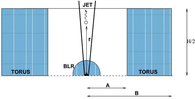
**Fig. 1.** Schematic AGN model (upper section) showing the broad-line spherical shell and the torus surrounding the central engine. The jet penetrates the BLR region on its way out of the central AGN.  $\gamma$ -rays originate at different positions along the jet.
