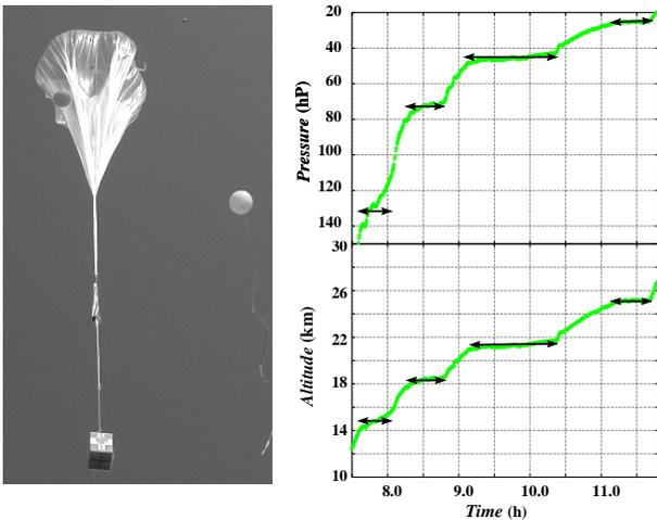
**Fig. 2.** The balloon payload picture just after the launching, and the flight curves
