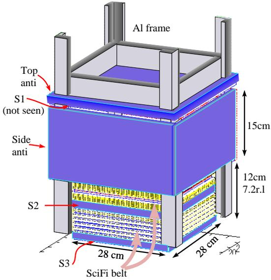
**Fig. 1.** Schematic view of BETS detector
