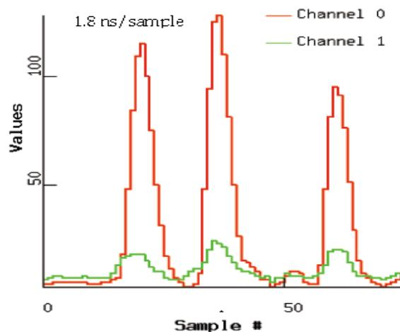
Figure 2. Waveform containing three separate photoelectrons, recorded by the ATWD.
