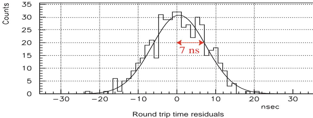
Figure 1. The residual values of round-trip times for time calibration pulses sent from the surface to the DOM, and from the DOM back to the surface. The round trip time is about 20  $\mu$ sec for a DOM in the middle of the string.
