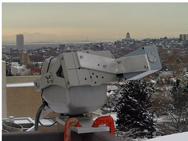
Fig. 4. The scanning cloud monitor in Salt Lake City during testing. Our IR detector views the sky through a fresnel lens limiting its FOV to a diameter of 3^\circ . The pan-and-tilt platform is computer controlled and we image the full sky every 12 minutes.
