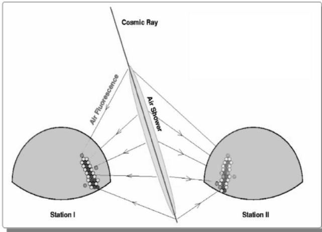
**Fig. 3.** An EAS appears as a line of illuminated pixels (PMTs) at each detector site. The line of the pixels determines the plane containing the detector and the EAS. For stereo observations, the intersection of the shower-detector planes from the two sites fixes the three dimensional geometry of the EAS.
