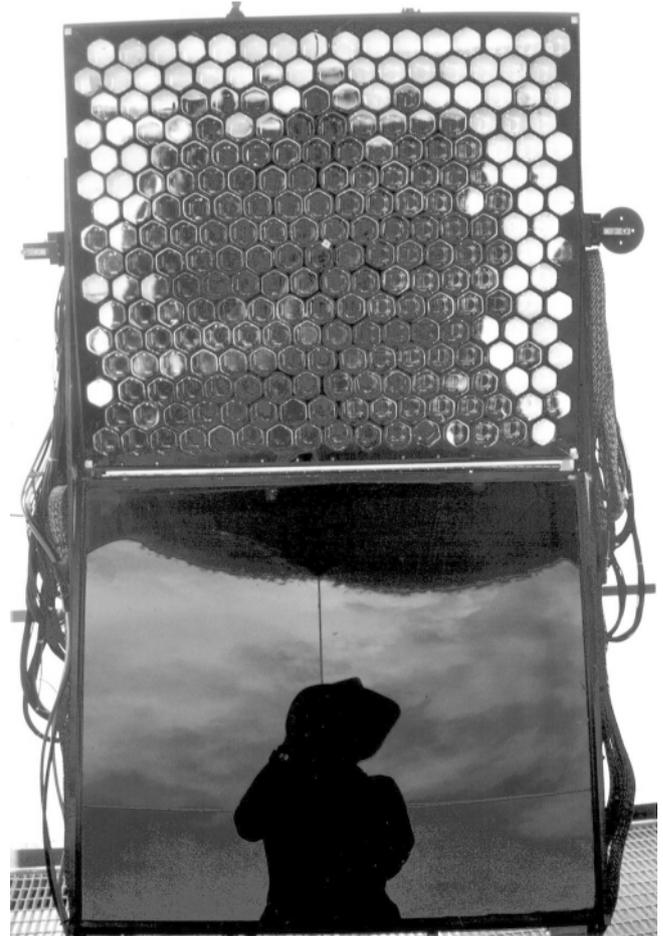
**Fig. 2.** A 256 pixel HiRes-I PMT cluster. The reflection of the photographer can be seen in the ultraviolet filter that has been swung open to expose the PMTs. The UV filter would normally cover the PMTs to filter out all but the 300-400 nm fluorescence light from the EAS.
