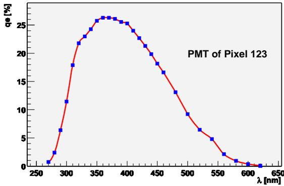
**Fig. 1.** quantum efficiency of the PMT for pixel 123
