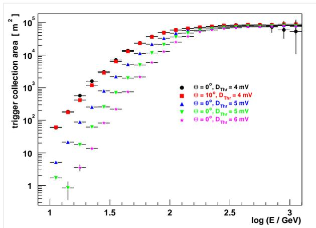
**Fig. 4.** The trigger collection area for gamma showers as a function of energy  $E$ .
