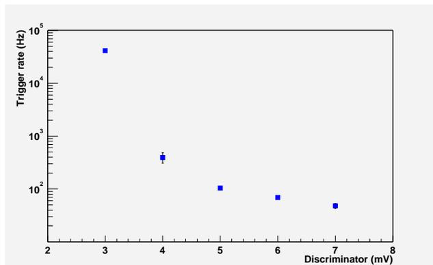
**Fig. 6.** Estimated trigger rates as a function of trigger discriminator for  $10^\circ$  zenith angle with 0.09 photo electrons of diffuse NSB and the Crab Nebula star field.
