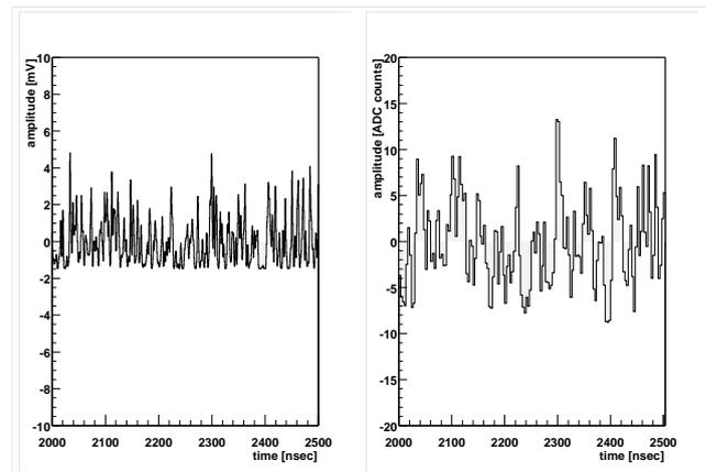
**Fig. 3.** The response of a pixel due to a star with magnitude  $m = 7$  in the field of view. On the left plot the analog signal that goes into the trigger system is plotted while on the right plot the content in the FADC system is shown.
