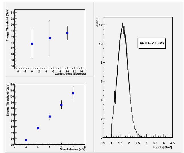
**Fig. 5.** On the left upper plot the energy threshold for different zenith angles is plotted while on the left bottom plot the energy threshold is plotted for several values of the trigger discriminator threshold. On the right plot a characteristic fit for  $dN/dE$  is shown (for showers at  $10^\circ$  with discriminator at 4 mV and diffuse NSB of 0.09 photo electrons per ns and pixel)
