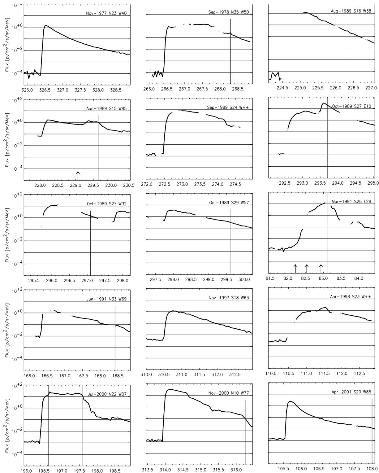
**Fig. 1.** Intensity time profiles as measured by the 48.0–96.0 MeV proton channel of the CPME instrument on board the IMP-8 spacecraft for 15 of the 21 SEP events described in Table 1.
