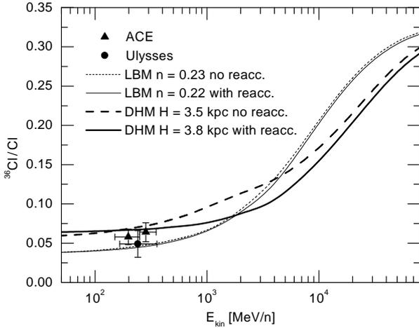
**Fig. 4.** The curves show the calculated  $^{36}\text{Cl}/\text{Cl}$ -ratio in the framework of the LBM and the DHM, with and without reacceleration. The curves are solar modulated with modulation parameter  $\Phi = 600$  MV. Data as in Figure 2, except for Ulysses: Connell et al. (1998).
