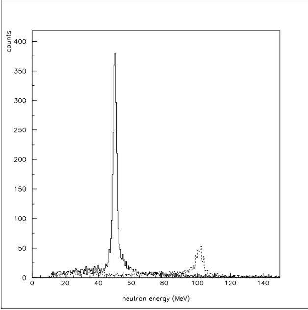
**Fig. 4.** GEANT4 simulated detection of 50 MeV (solid line), and 100 MeV (dashed line) neutrons by a  $10 \times 10 \times 10 \text{ cm}^3$  SONTRAC in the double  $np$  elastic scattering mode. For each energy 500000 events were processed.
