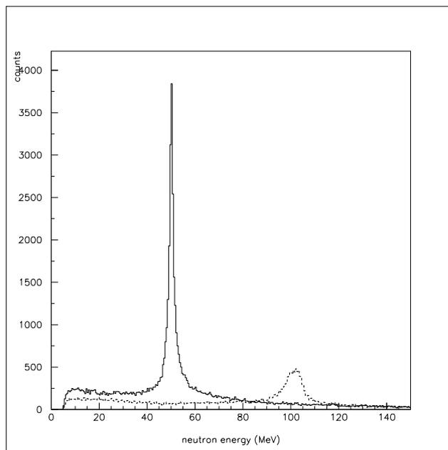
**Fig. 3.** GEANT4 simulated detection of 50  $MeV$  (solid line), and 100  $MeV$  (dashed line) neutrons by a  $10 \times 10 \times 10 cm^3$  SONTRAC in the single  $np$  elastic scattering mode. For each energy 500000 events were processed.
