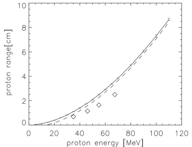
**Fig. 1.** GEANT4 computed proton range of a scintillating material with the same density and composition as the SONTRAC scintillating fibers (solid lines). The dashed line is obtained when the proton beam crosses first an aluminum layer of 1mm. The diamonds represent measurements with the SONTRAC scientific model.
