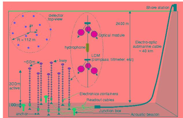
Fig. 1. Figure 1. The ANTARES 0.1 km<sup>2</sup> detector concept.
