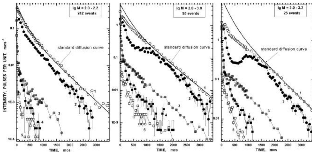
Fig. 3. Averaged temporal intensity distributions of pulses registered from the neutron detectors of “B” and “D” monitor units. From top to bottom: 1 – SNM15 neutron counters of the “B” monitor unit, 2 – SNM15 of unit “D”, 3 – internal SNM18 counters of unit “B”, 4 and 5 – external SNM18 of units “D” and “B” correspondingly.
