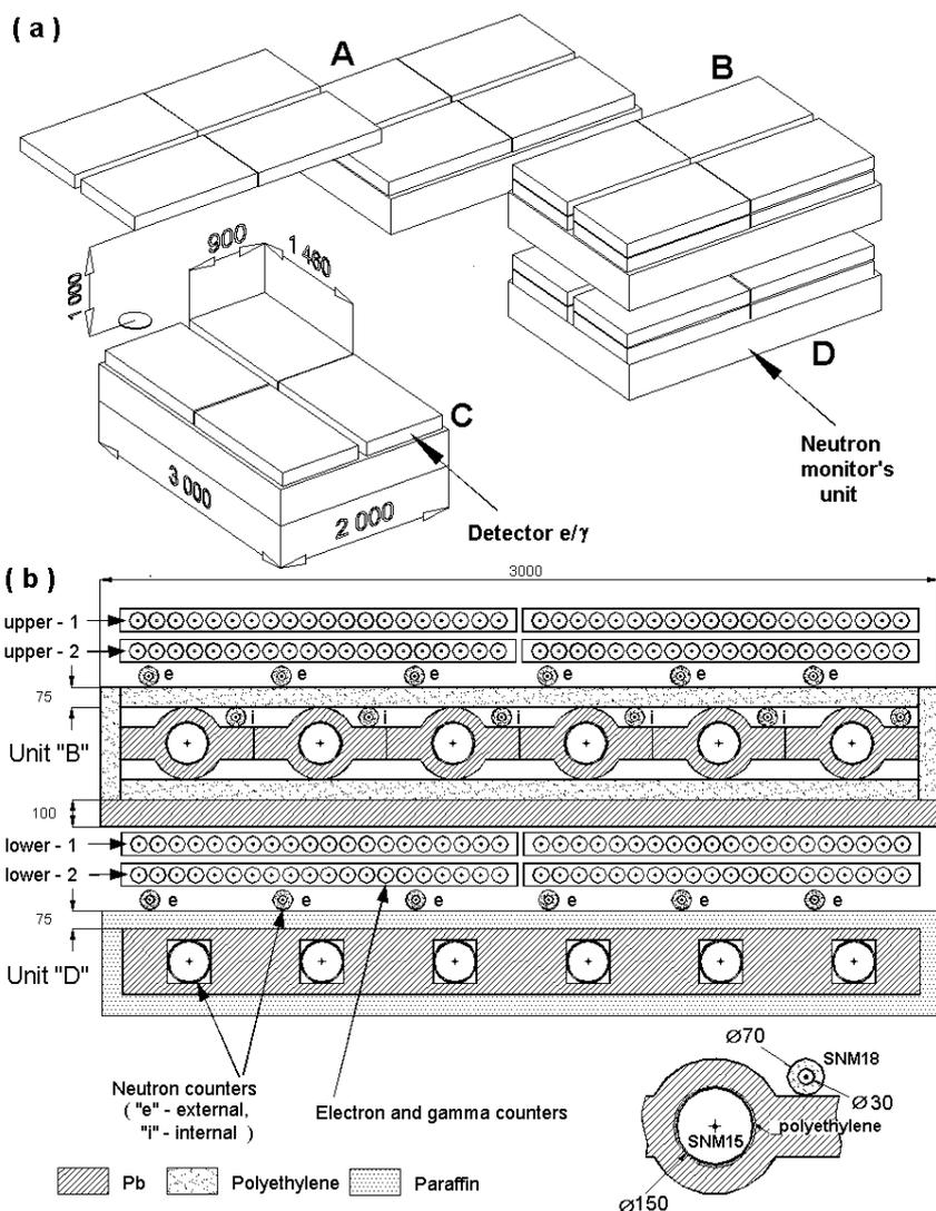
Fig. 1. General layout of the four neutron monitor's units (a) and the cross-section of units "B" and "D" (b).
