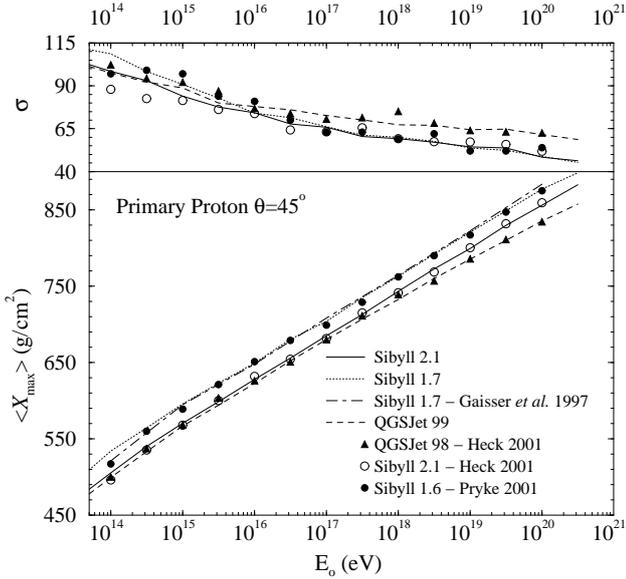
**Fig. 2.** Average depth of maximum  $\langle X_{\max} \rangle$  of proton showers as a function of primary energy generated by our one dimensional method and CORSIKA code using different hadronic interaction models. The top panel shows the corresponding sigma values.
