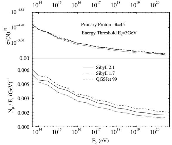
**Fig. 5.** Number of muons at sea level with energy above 3 GeV. The numbers have been normalized to primary energy. The top panel shows the statistical errors.
