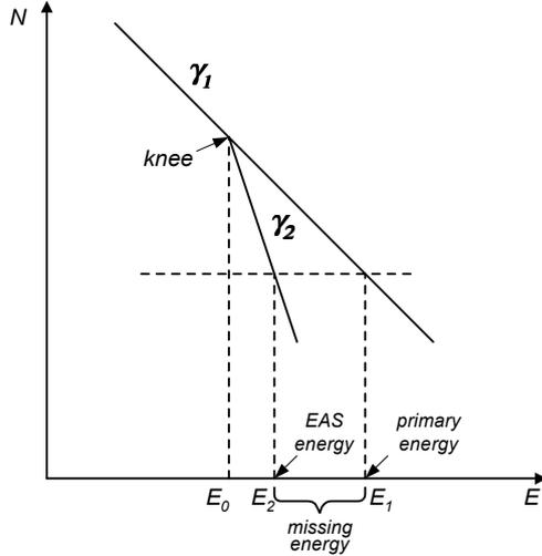
Fig. 1. Missing energy definition.
