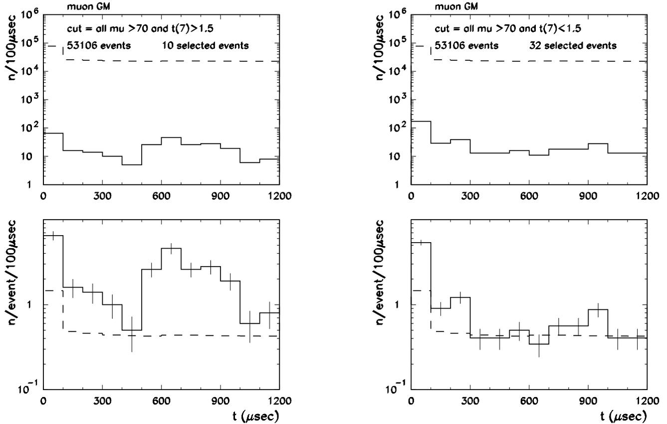
**Fig. 2.** Time distributions of the number of hit G-M counters: broken line – all events, solid line – events with the threshold of 70 hit muon blocks. Upper figures are histograms, lower are recalculated per 1 event. Solid lines on left figures with 2 or more signals in 600–700  $\mu\text{s}$  interval, on right figures – with 0 or 1 signal in the same interval.
