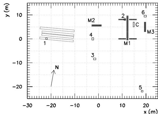
**Fig. 1.** Schematic plan of the Lodz air shower array. Scintillation counters are denoted by numbers.
