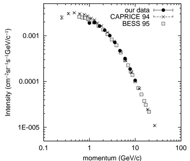
Fig. 1. Muon momentum spectrum in vertical at sea level.
