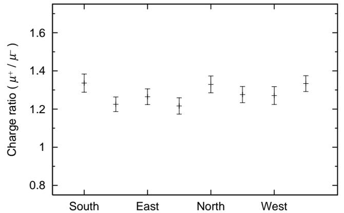
**Fig. 5.** The azimuthal angular dependence of the muon charge ratio at zenith angle  $40^\circ$  in momentum region,  $3.0 \sim 10.0 \text{ GeV/c}$ .
