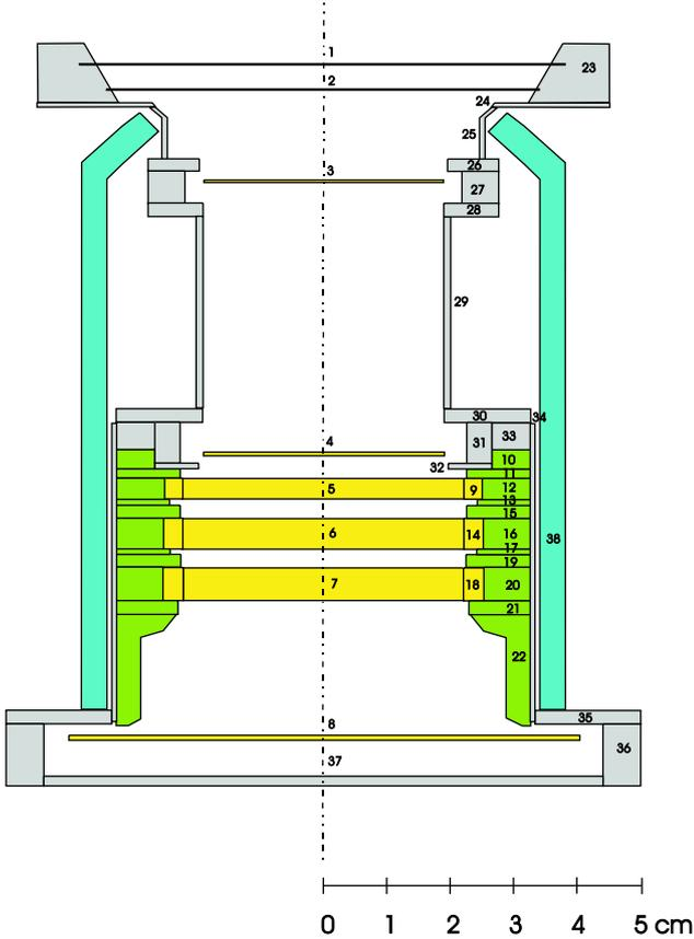
**Fig. 1.** EPHIN sketch showing the 38 sections introduced in the Monte Carlo simulation.
