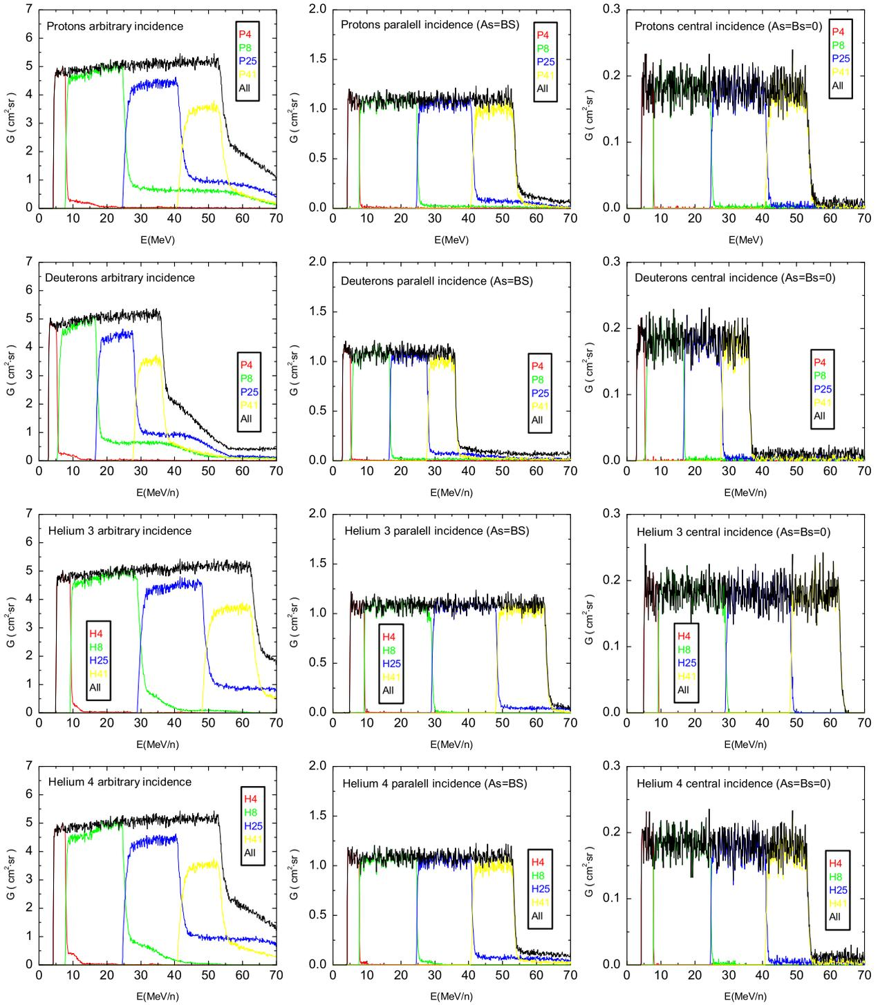
**Fig. 4.** Dependence on the energy of geometrical factors for protons, deuterons,  $^3\text{He}$  and  $^4\text{He}$  in  $\text{cm}^2 \cdot \text{sr}$ .
