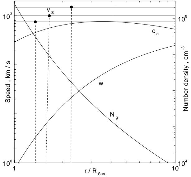
**Fig. 1.** Solar wind ( $w$ ), Alfvén wave ( $c_a$ ) and shock ( $V_s$ ) speeds and gas number density  $N_g$  as a function of heliocentric distance. Vertical dashed lines shows the position of the shock where it becomes inefficient accelerator.
