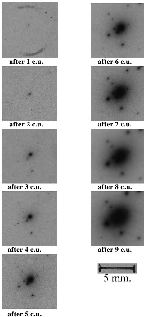
**Fig. 3.** Halo images in various layers X-ray film in the calorimeter from 1 c.u. to 9 c.u.
