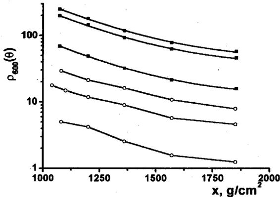
Figure 1. Shower development curves. Solid squares - reconstructed curve. Empty circles - experimental data (Efimov et al., 1991).
