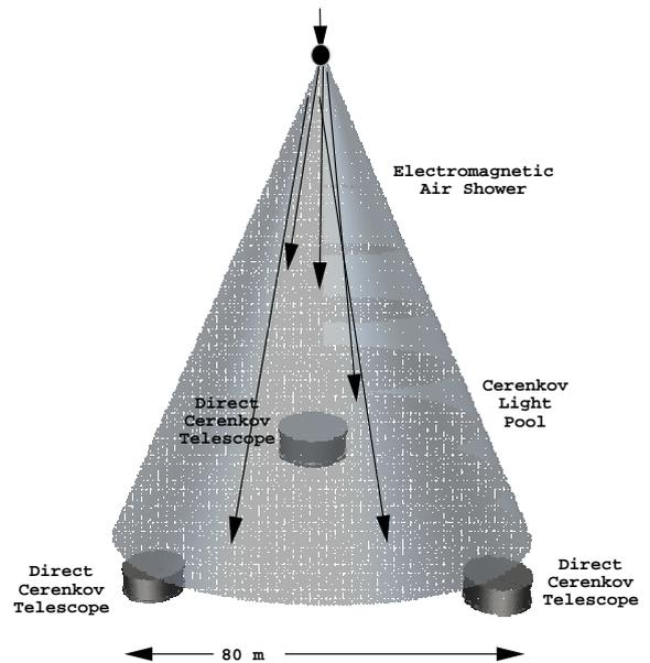
**Fig. 3.** Conceptual Direct Čerenkov Observatory General design. Each wide field of view ( $45\text{-}60^\circ$ ) DČO telescope observes the Čerenkov light pool from the cosmic ray air shower with  $0.1^\circ$  pixels. The telescopes are nominally separated by a distance of 80 m.
