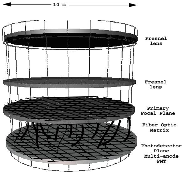
**Fig. 4.** Conceptual Direct Čerenkov Observatory telescope structure. The UV transmitting Fresnel lenses provide the wide field of view ( $45\text{--}60^\circ$ ) for the instrument. Pixels in the focal plane are optically multiplexed to the photomultiplier readout plane to reduce cost.
