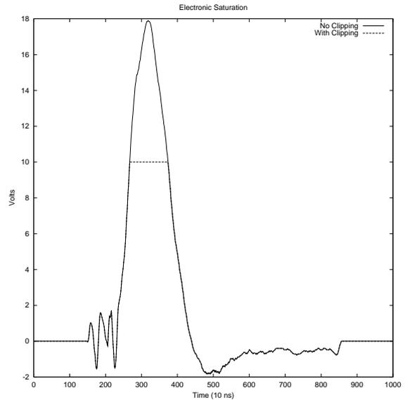
**Fig. 3.** Wave Forms are Clipped at 10 Volts
