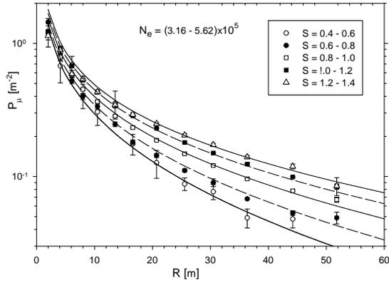
**Fig. 2.** Muon lateral distribution for different age parameters and  $N_e = (3.16 - 5.6) \cdot 10^5$
