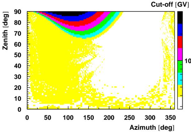
**Fig. 2.** The directional dependence of the geomagnetic cut-off for Fort Sumner, New Mexico ( $34.3^\circ$  North,  $104.1^\circ$  West). The counting of the azimuth angle  $\phi$  follows the convention used by the Super-Kamiokande detector,  $\phi = 0^\circ$  means looking to the South,  $\phi = 90^\circ$  to East, etc.
