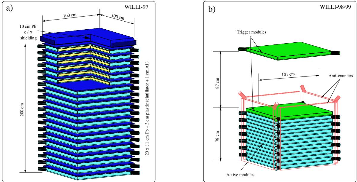
**Fig. 2.** a) The original sampling calorimeter configuration of the WILLI detector used in WILLI-97 runs. b) The second configuration, improved for the measurements on the muon charge ratio used in WILLI-98 and WILLI-99 runs.
