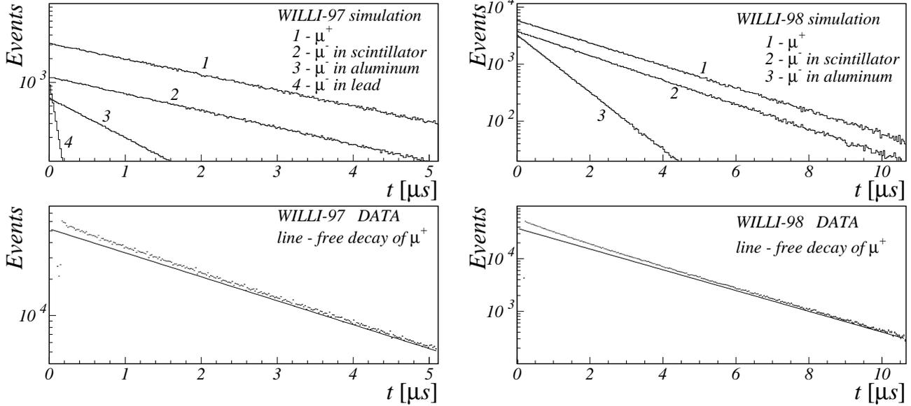
**Fig. 3.** Upper figures: Monte Carlo simulation results on the contribution of different absorber materials to the total decay curve, assuming  $N(\mu^+)/N(\mu^-) = 1$ . Lower figures: The experimental decay curves compared with the free decay of positive muons.
